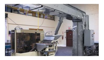
The sorter receives product from the customer's metal detector on the end of the molding plant line and transfers the product to another Eriez feeder to transfer the product to the elevator/conveyor.
